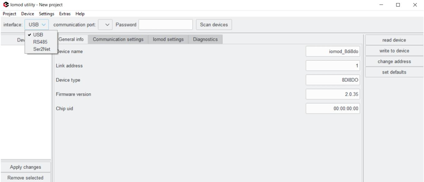
The user can either configure devices online or offline. This means configuration is possible without directly connecting to IOMOD and can be done using templates. The templates allow the creation of configurations for one device or a whole set of IOMODs. By connecting IOMODs to a ser2net device, they can be configured remotely. This also includes firmware upgrades, configuration and diagnostics. More configuration information will be mentioned in the configuration chapter.
