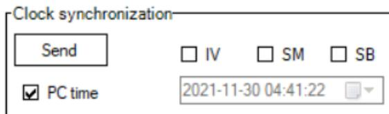
If "PC time" checkbox is checked, then the PC time will be sent. If it's not checked user can set time manually.
