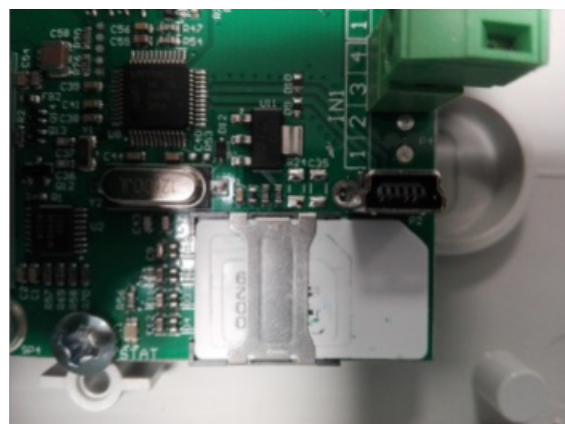
SIM card connection diagram
