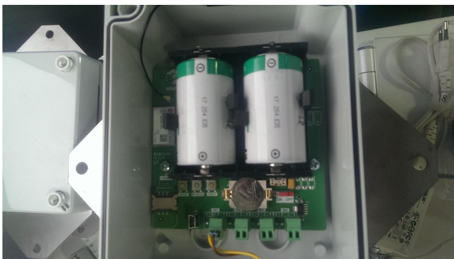
MV Beacon B+ power pin and battery layout
