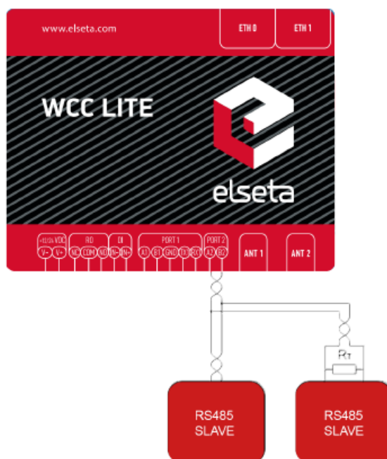
Figure 8: Typical WCC Lite RS-485 connection diagram
