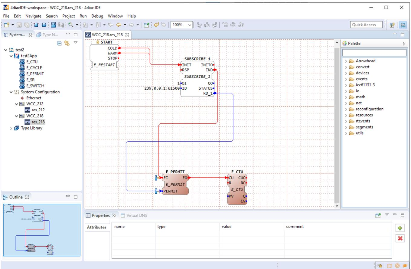
To count the blinking, two new Function Blocks (FBs) have been added to the existing application for a different device (WCC\_218):
