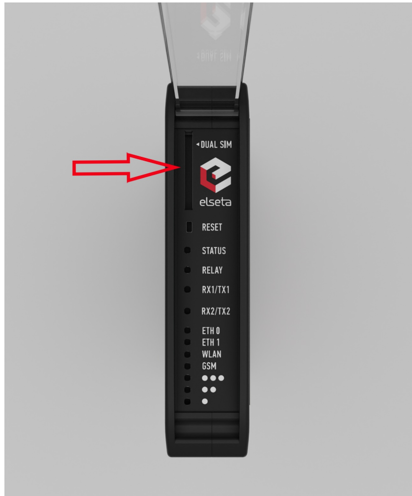
Figure 5: WCC Lite Dual-SIM card slot
