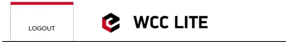
To log out of the device graphical user interface a logout button in interface's upper right corner should be pressed. A user is automatically disconnected after ten minutes of inactivity. This ensures that the device would not be suspect to any deliberate damage made by unauthorized access.
