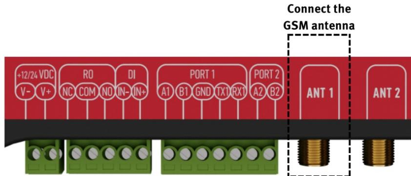
Connect an antenna to the SMA connector labeled “ANT1”. Select a good antenna placement spot considering the operation environment and network coverage of your mobile provider in the area. To enable MIMO functionality for 4G (LTE) modems a second antenna should be connected to the SMA connector labeled “ANT2”.
