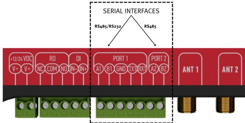
WCC Lite RS485 interface supports baud rates up to 115200 and has an integrated 120 termination resistor. It is recommended to use termination at each end of the RS485 cable. To reduce reflections, keep the stubs (cable distance from main RS485 bus line) as short as possible when connecting device. See typical RS485 connection diagram on figure 8.
