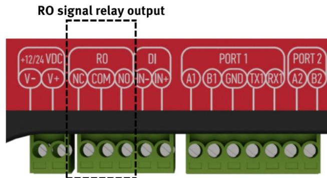
Maximum switching power is 60W, maximum contact current is 2A, maximum switching voltage is 60VDC/60VAC. The lower is switching power, the higher is lifecycle of Relay Output.
