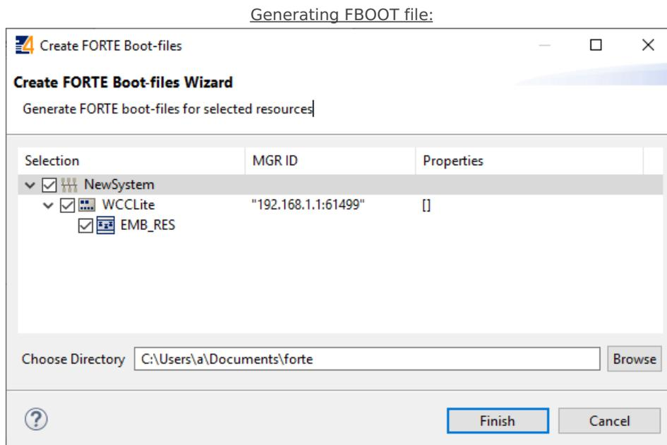
Upload button for FORTE file in web interface can be found in Protocol Hub tab, Configuration screen (FORTE boot file upload supported for versions v1.4.0 and above). You should see a view as in picture below.
