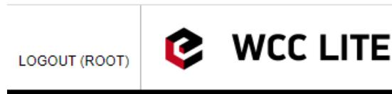
To log out of the device graphical user interface a logout button in the interface's upper right corner should be pressed. A user is automatically disconnected after ten minutes of inactivity. This ensures that the device would not be suspect to any deliberate damage made by unauthorized access.
