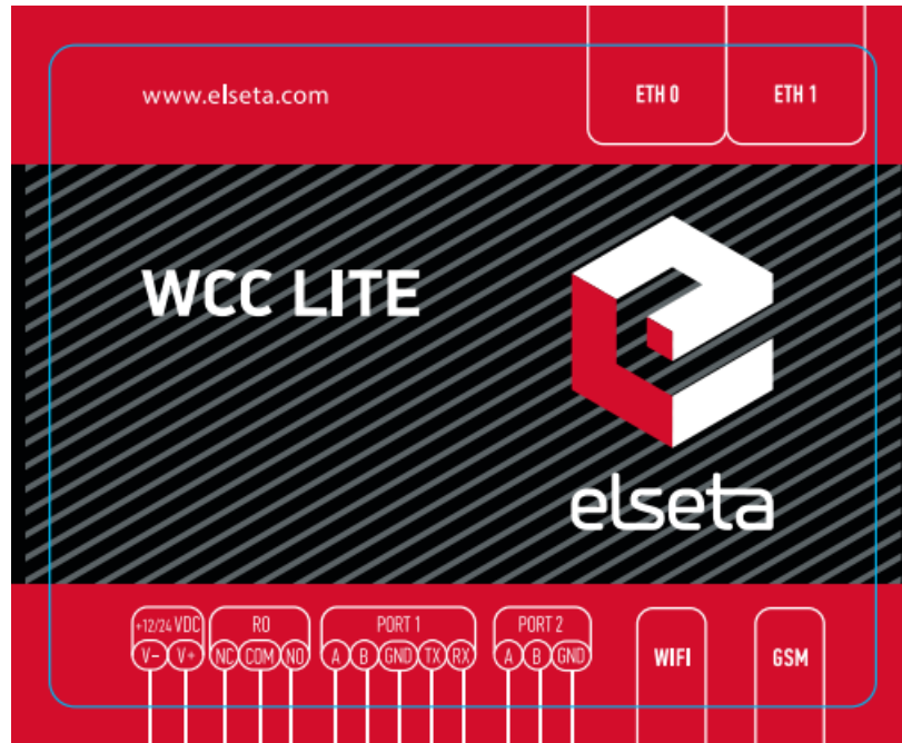
Figure 1. Wi-Fi antenna connector (hardware version older than 1.4 )
