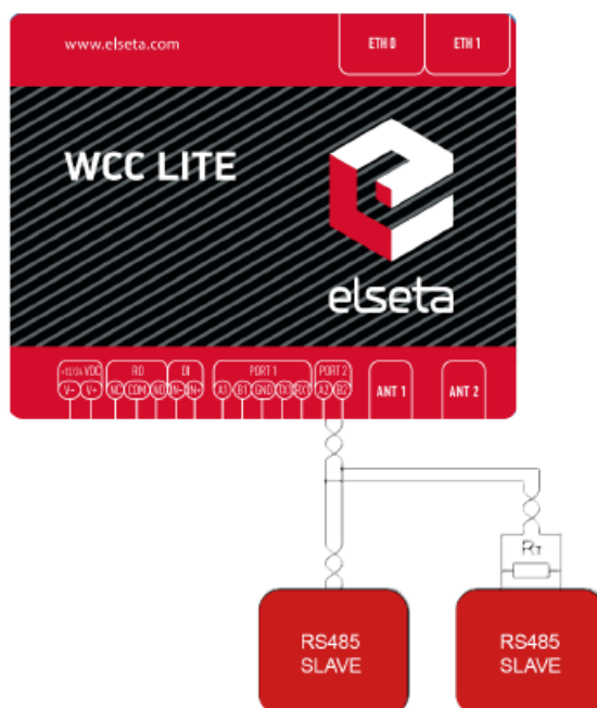
Figure 8: Typical WCC Lite RS-485 connection diagram
