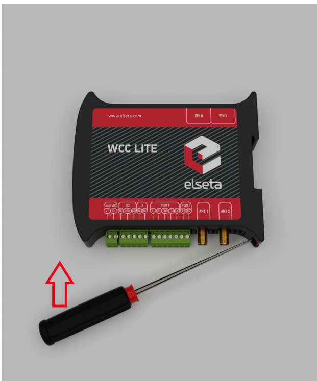
Figure 2: WCC Lite DIN rail mounting clip
