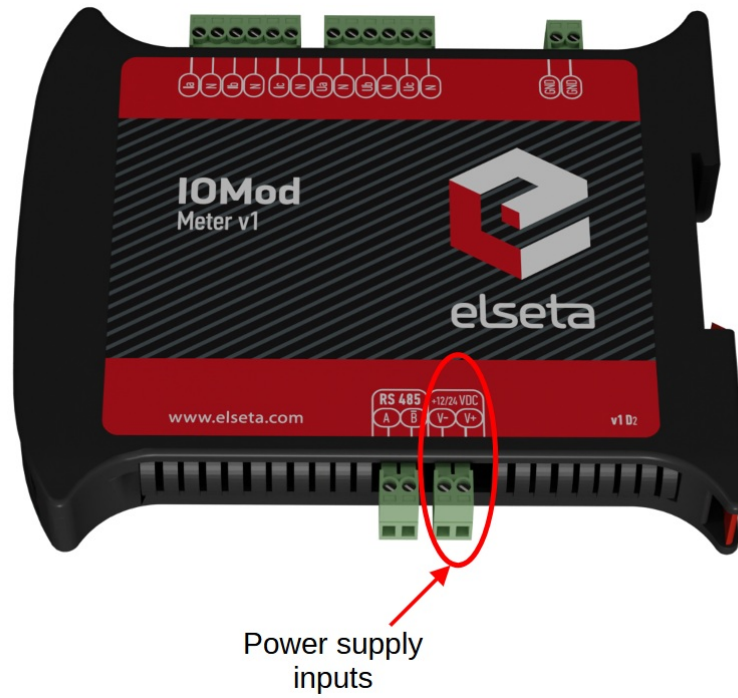
Fig. 4.3.1. Power supply inputs physical location
