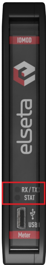
Fig. 2.3.1. IOMod Meter LEDs physical location
