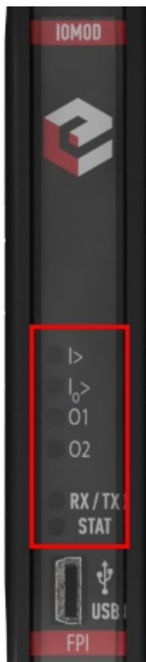
Fig. 2.3.1. IOMod FPI LEDs physical location
