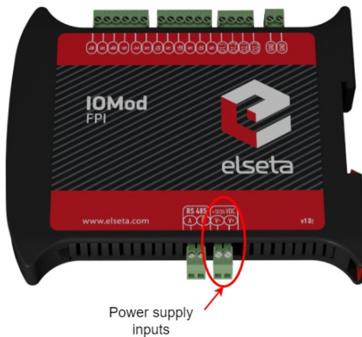
Fig. 4.4.1. Power supply inputs physical location
