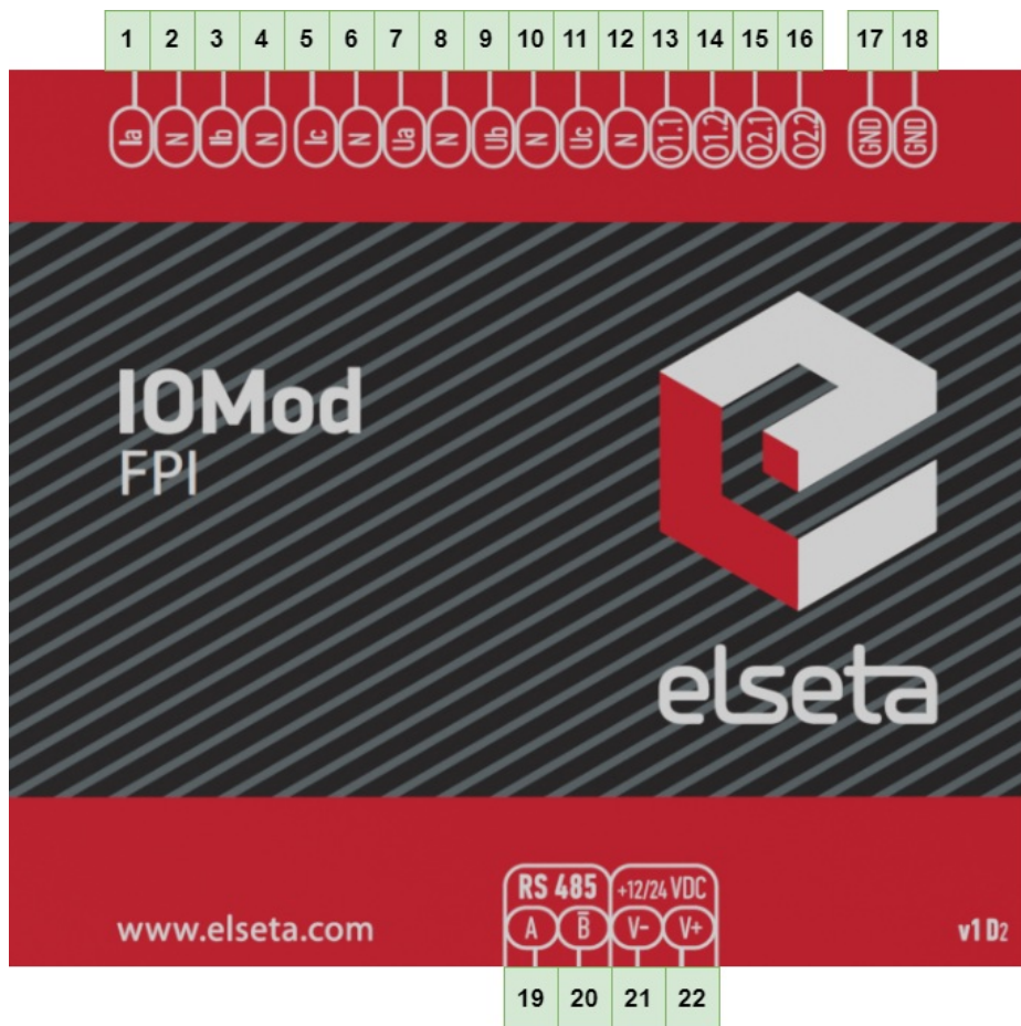
Fig. 2.2.1. IOMod FPI terminal diagram
