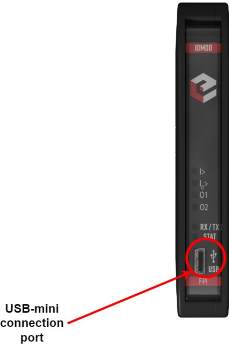
Fig. 4.5.2. IOMod FPI USB connection port physical location
