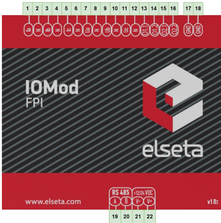
Fig. 2.2.1. IOMod FPI terminal diagram
