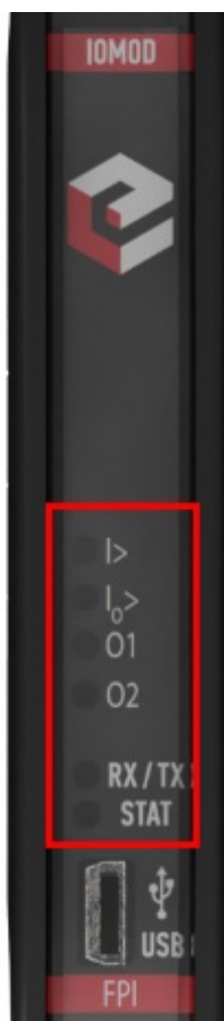
Fig. 2.3.1. IOMod FPI LEDs physical location
