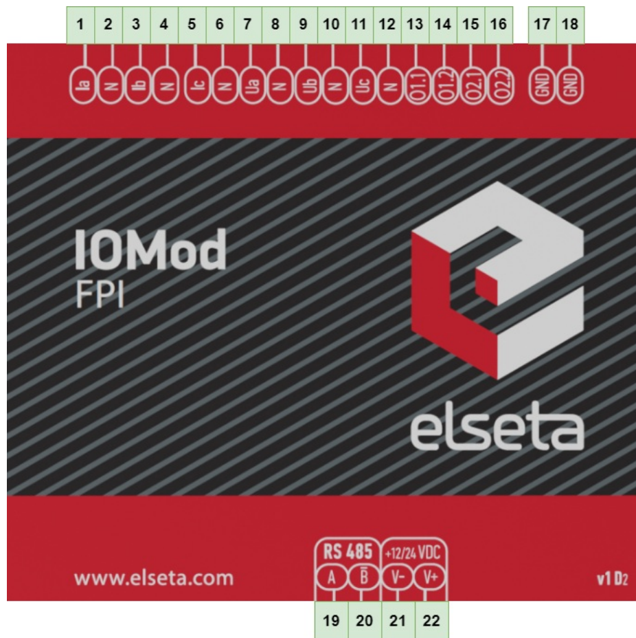
Fig. 2.2.1. IOMod FPI terminal diagram
