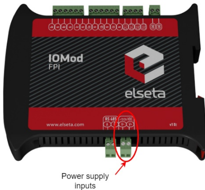
Fig. 4.4.1 Power supply inputs physical location
