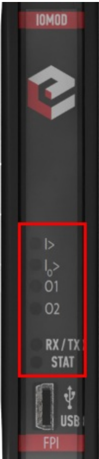
Fig. 2.3.1 IOMod FPI LEDs physical location
