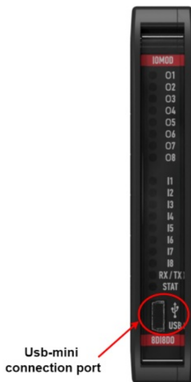
Fig. 4.4.2. IOMod 8DI8DO USB connection port physical location
