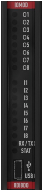
Fig. 2.3.1 IOMod 8DI8DO LEDs physical location
