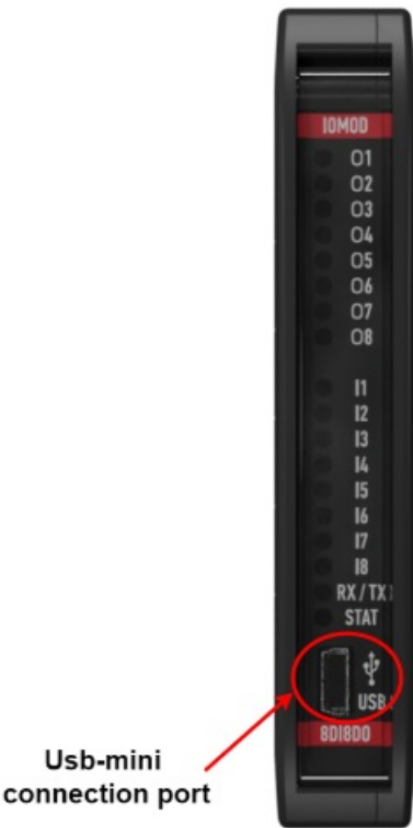
Fig. 4.3.2. IOMod 8DI8DO USB connection port physical location
