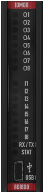
Fig. 2.3.1 IOMod 8DI8DO LEDs physical location
