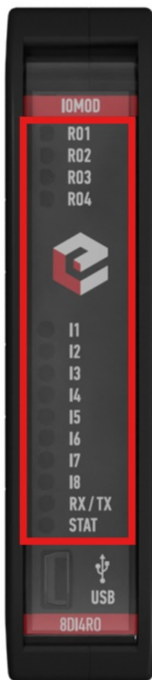
Fig. 2.3.1 IOMod 8DI4RO LEDs physical location
