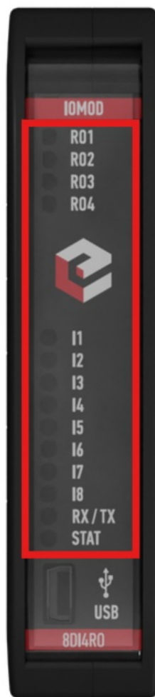
Fig. 2.3.1 IOMod 8DI4RO LEDs physical location
