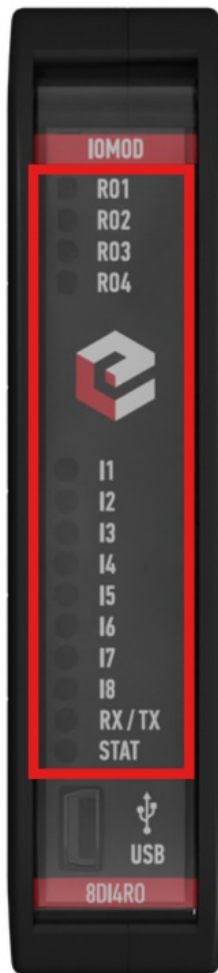
Fig. 2.3.1 IOMod 8DI4RO LEDs physical location
