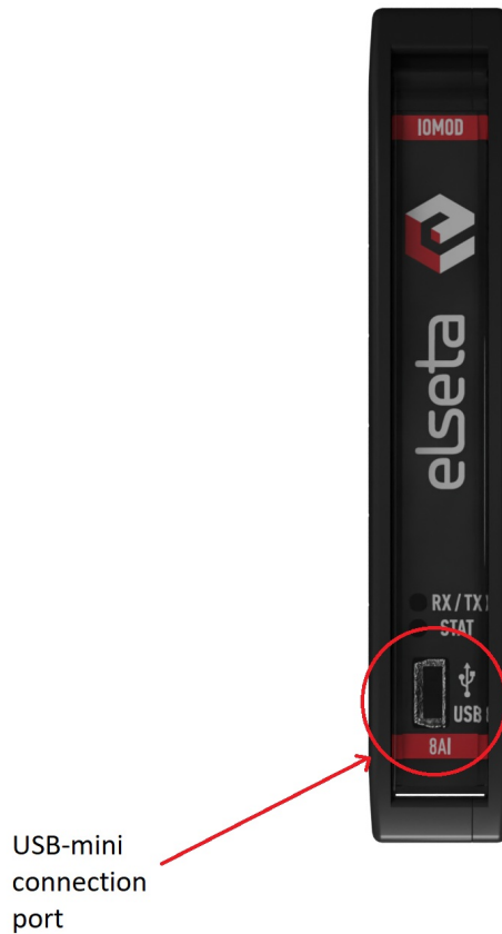
Fig. 4.3.2 IOMod 8AI USB connection port physical location
