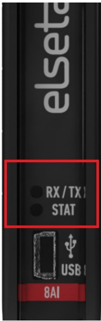
Fig. 2.3.1 IOMod 8AI LEDs physical location
