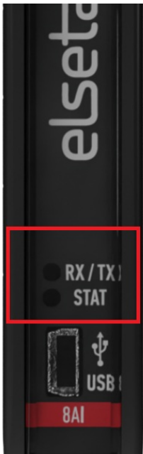
Fig. 2.3.1 IOMod 8AI LEDs physical location
