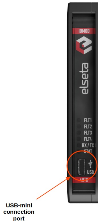
Fig. 4.4.2. IOMOD 4RTD USB connection port physical location
