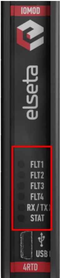
Fig. 2.3.1 IOMod 4RTD LEDs physical location
