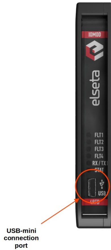
Fig. 4.3.2 IOMod 4RTD USB connection port physical location
