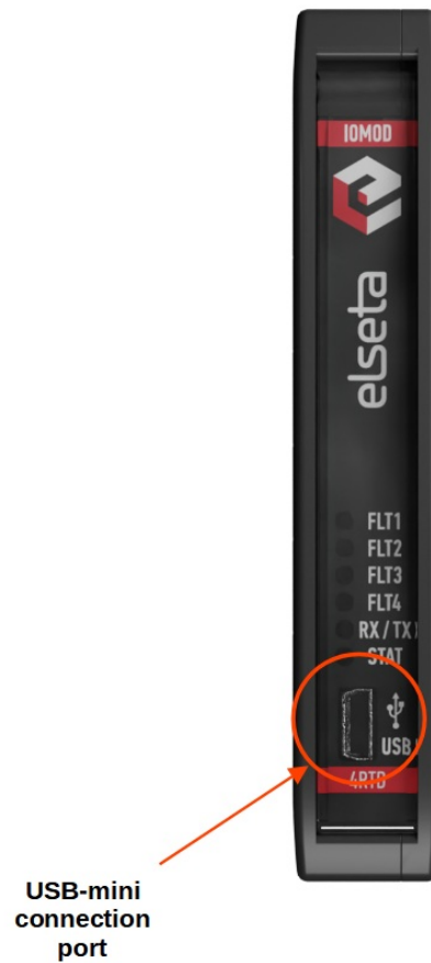
Fig. 4.3.2 IOMod 4RTD USB connection port physical location
