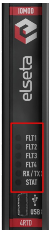
Fig. 2.3.1 IOMod 4RTD LEDs physical location
