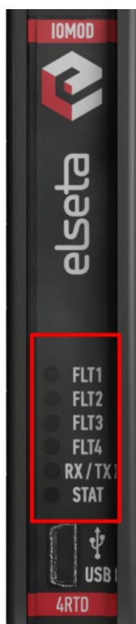
Fig. 2.3.1 IOMod 4RTD LEDs physical location
