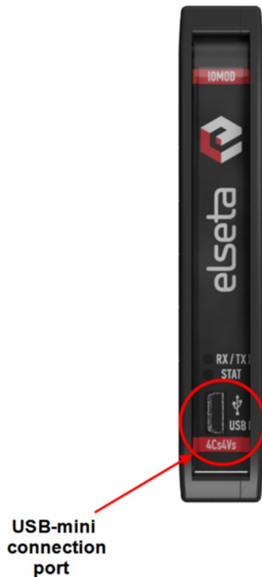
Fig. 4.4.2 IOMod 4Cs4Vs USB connection port physical location
