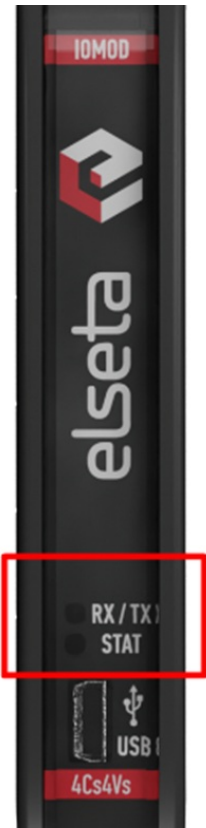
Fig. 2.3.1 IOMod 4Cs4Vs LEDs physical location
