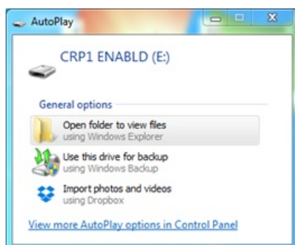
Fig. 10.1. Reconnecting as a mass storage device
