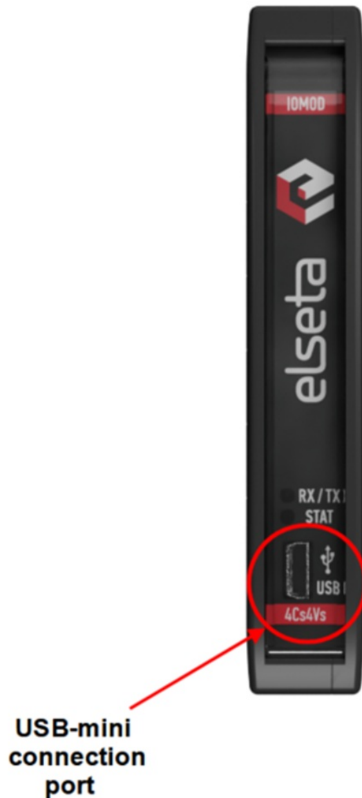
Fig. 4.4.2 IOMod 4Cs4Vs USB connection port physical location
