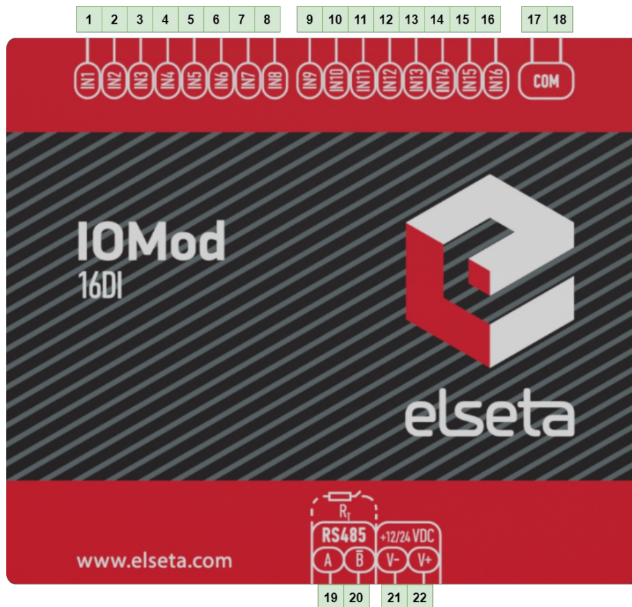
Fig. 2.2.1 IOMod 16DI terminals diagram
