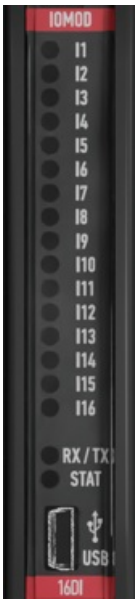
Fig. 2.3.1 IOMod 16DI LEDs physical location
