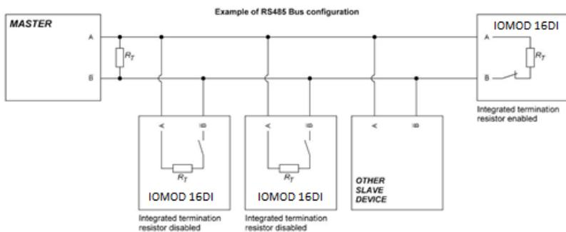
IOMOD 16DI has 1/8 Unit load receiver which allows to have up to 256 units on line (compared to standard 32 units). To reduce reflections, keep the stubs (cable distance from main RS485 bus line) as short as possible when connecting device.
