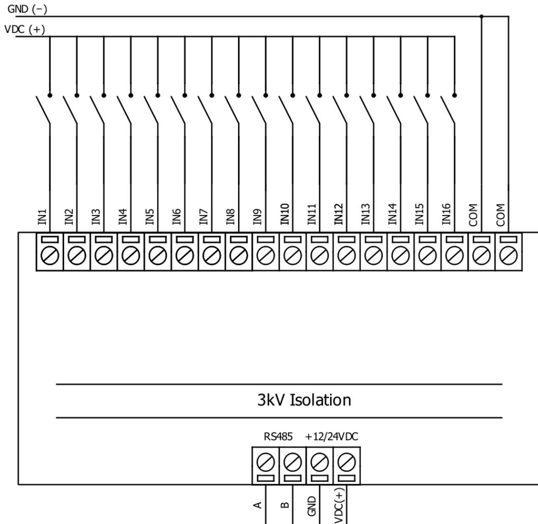
User also can configure to enable pull-up resistors (function is applied for all inputs) and software input inversion. With this configuration, user will see inputs connected to 0V (see Fig. 5.3) as “high” or state “1”, input status LED will NOT glow
