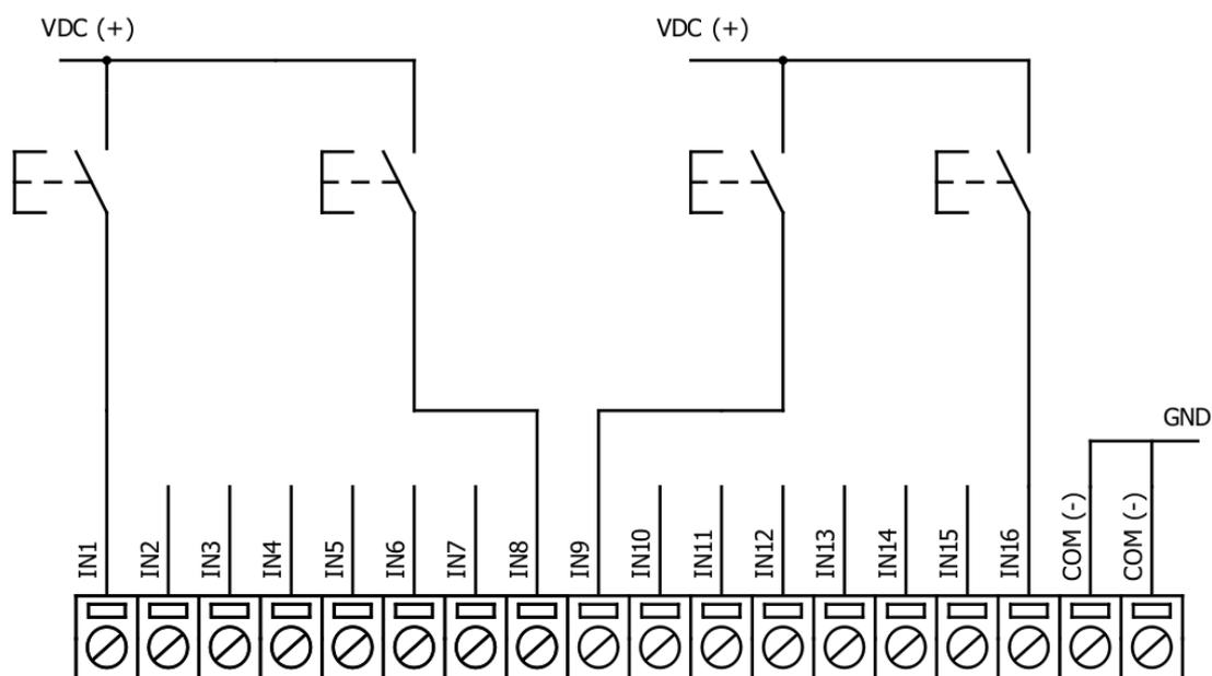
In addition to this, Fig. 3.2 shows 1<sup>st</sup> + 2<sup>nd</sup> and 11<sup>th</sup> + 12<sup>th</sup> inputs are grouped into pair. Now, General Interrogation will be composed of 14 input states (with IN2 and IN12 missing). Input numbers is represented by “Info number” in protocol. Here, COM is connected to positive voltage of power supply and inputs are controlled by negative voltage.
