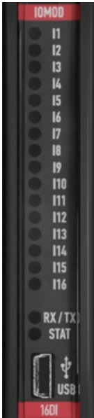
Fig. 2.3.1 IOMod 16DI LEDs physical location
