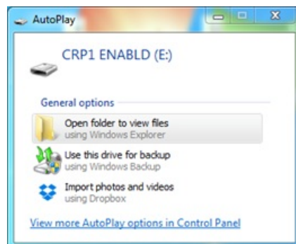
Fig. 6.5. Reconnecting as a mass storage device
