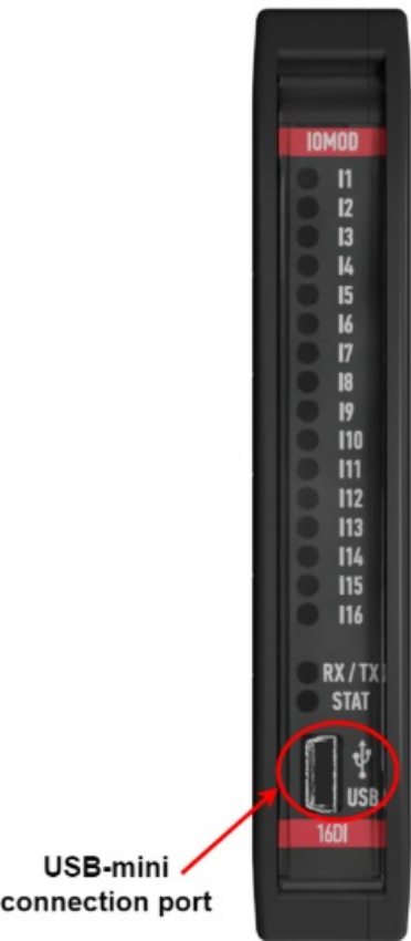
Fig. 4.4.2. IOMod 16DI USB connection port physical location
