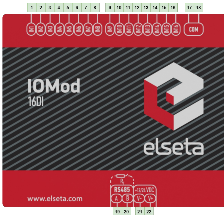
Fig. 2.2.1 IOMod 16DI terminal diagram
