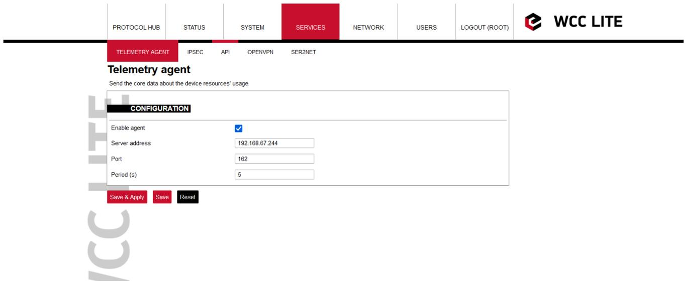
After setting up the Telemetry agent tab navigate to Network -> Firewall -> Traffic rules. Enable the Allow-SNMP packet and edit the destination port to match the one in Telemetry agent screen (for this example it is 162):
