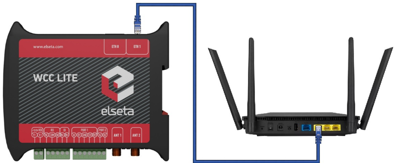
Fig. 4 Wcc Lite's ETH1 port connected to the internet router for internet access
