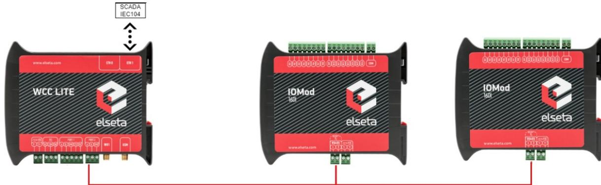
Typical connection schematic for two IOMod 16DI
