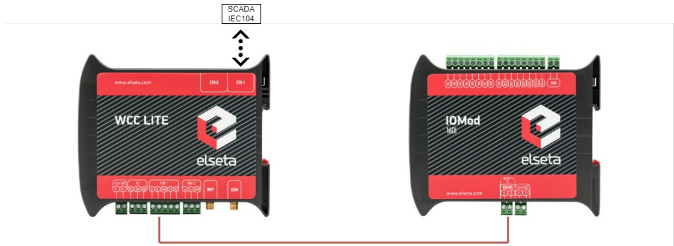
Typical connection schematic for IOMod 16DI
