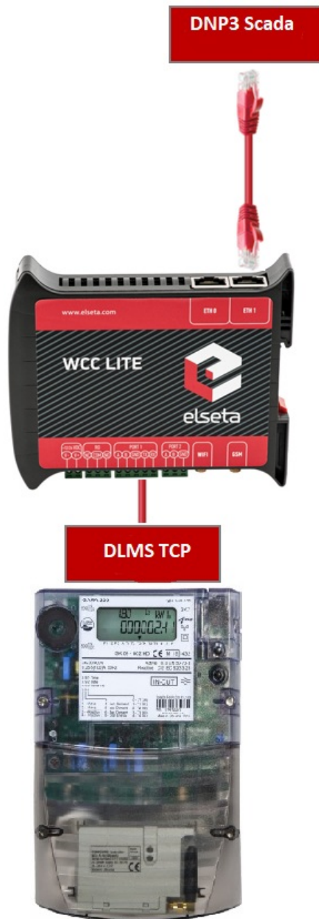
Fig 1. Connection scheme.
