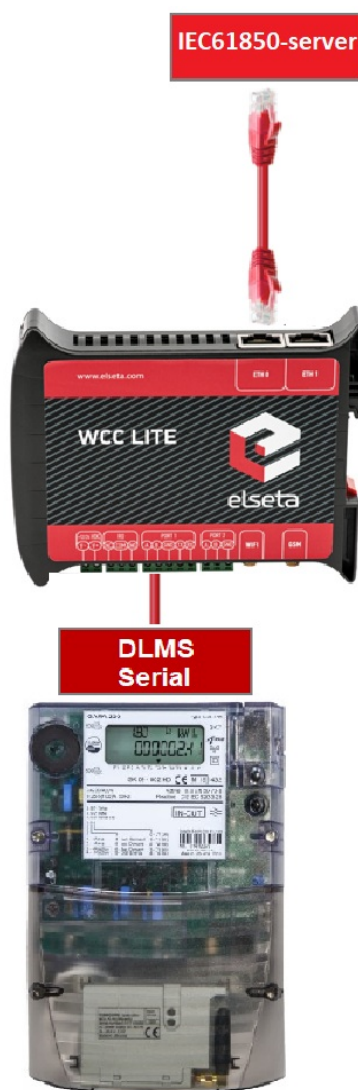
Fig 1. Connecting Meter with DLMS serial protocol to WCC Lite and IEC61850 server
