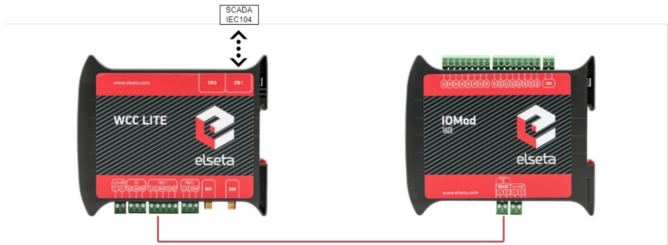
Typical connection schematic for IOMod 16DI
