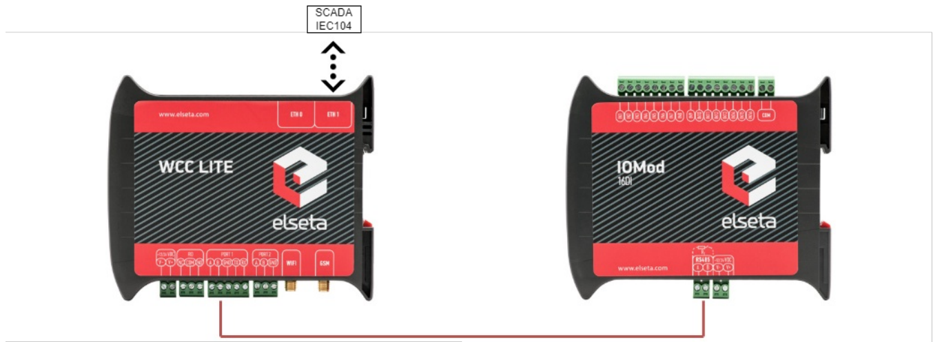
Typical connection schematic for IOMod 16DI
