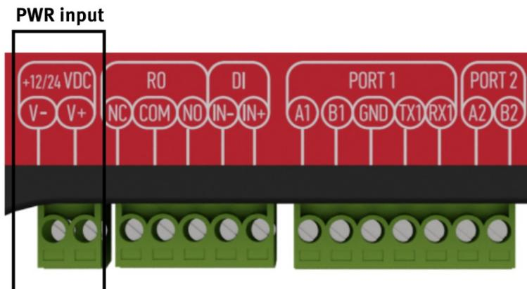
**⚠ Note:** Make sure that device is compatible with your power source before proceeding! Check the label next to power connector or on the side of device.
