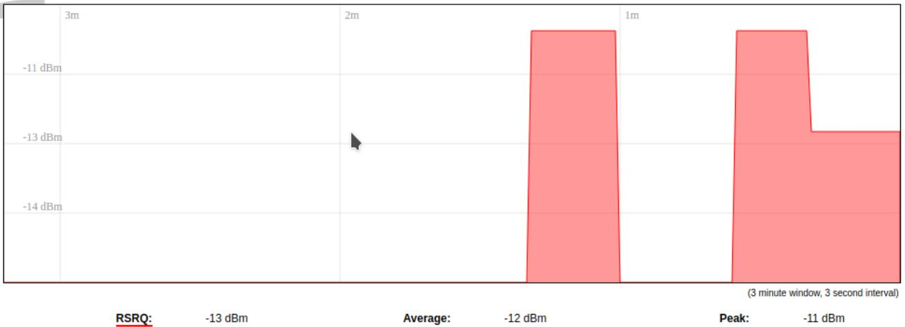
Graph representation of gsm modem receiving signal quality. RSRP - RSRQ graph is showed, when connected to 4G/LTE network, RSSI - when 2G/3G networks are used.
