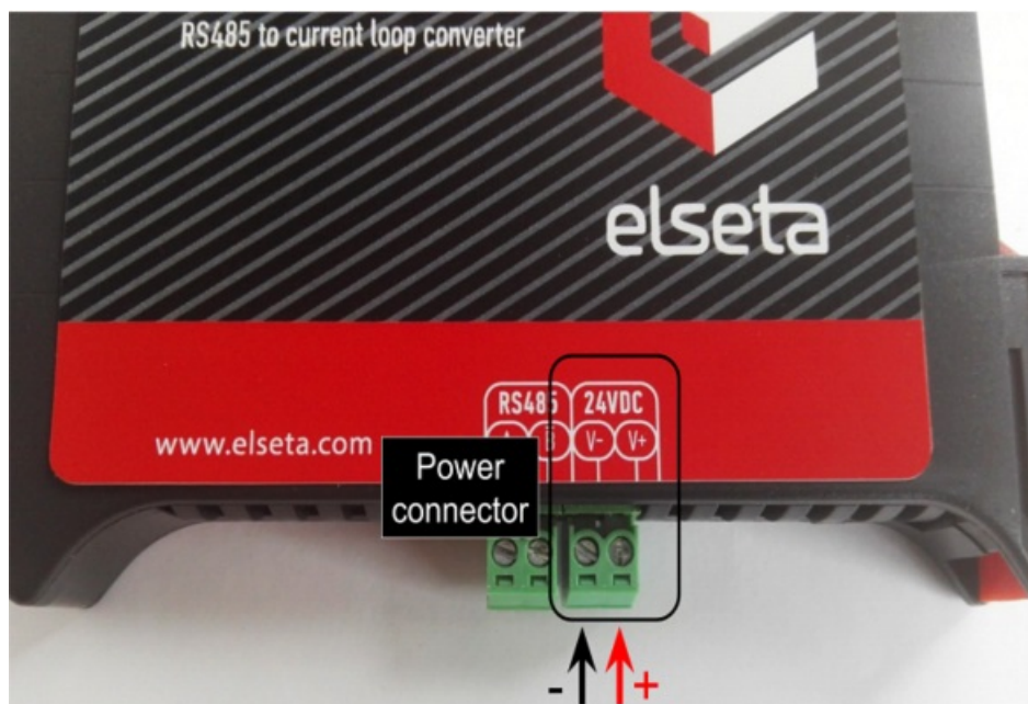
Fig 2. Power connector
