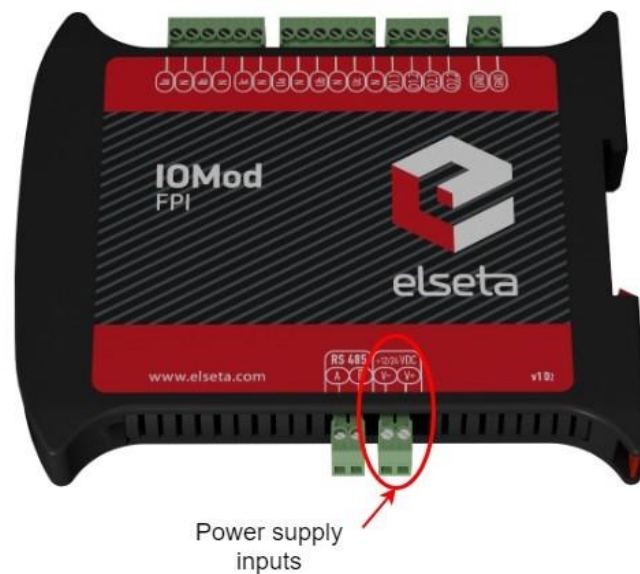
Fig. 4.4.1. Power supply inputs physical location
