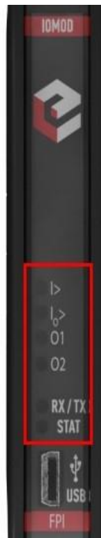
Fig. 2.3.1. IOMod FPI LEDs physical location
