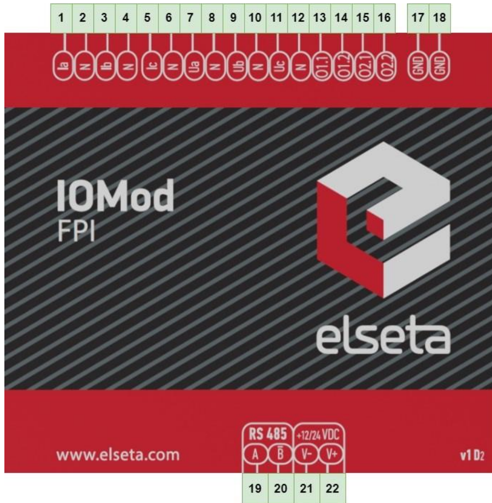
Fig. 2.2.1. IOMod FPI terminal diagram
