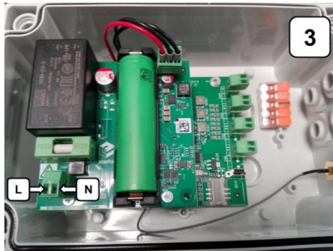
First, connect the three-wire cable as shown in steps 1-2 of the power connection instructions. Using a 2-wire cable, connect the unit's AC power as shown in step 3 of the connection instructions. Turn on the automatic power switch only when all the work of connecting the device has been completed (SIM card inserted, input cables connected).
