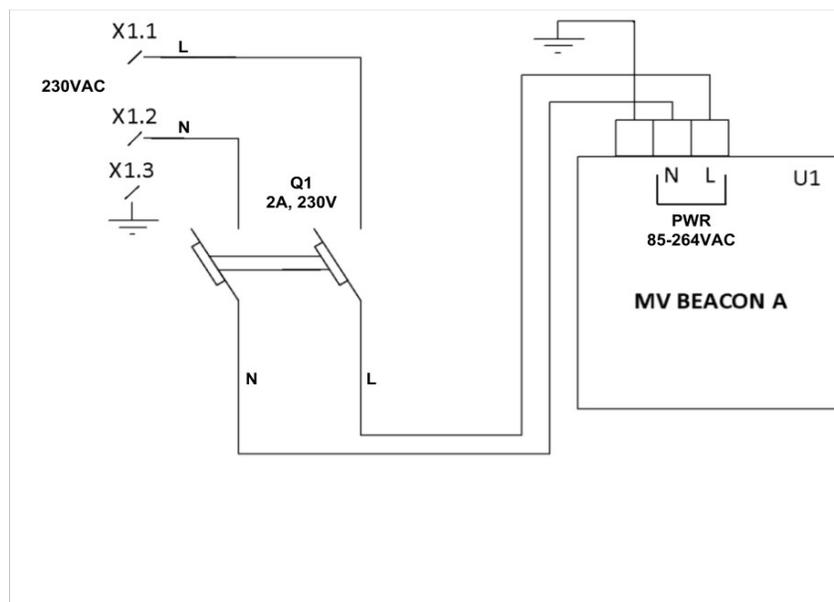
Recommended MV BEACON A power connection diagram
