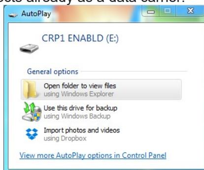
The user must delete the existing firmware.bin file and load the new one by copying.
