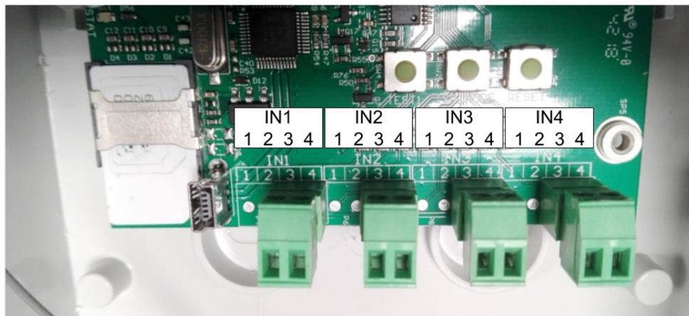
Input contacts 3 and 4 are used to connect the input signal. Methods of transmitting external signals to MV BEACON:
