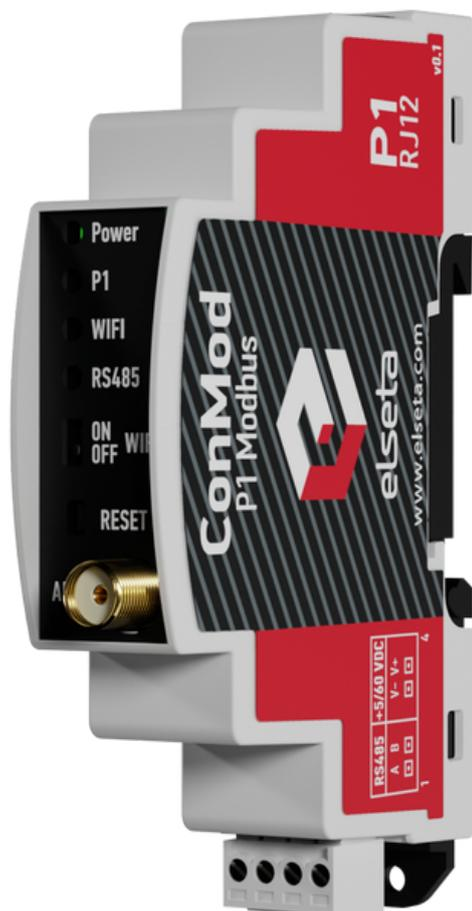
ConMod P1Modbus is a small-size industrial protocol converter for smart Meters with P1 interface output to convert meter data into industrial standard protocols Modbus RTU and Modbus TCP with interfaces RS485 and Wi-Fi (2,4GHz).
