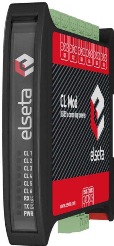
CLMod is an RS485 to 20 mA current loop converter. CLMod can remotely gather data from electricity meters. This converter was developed to read multiple meters of data over a 20mA current loop interface with long-distance lines up to 2km. CLMod with 6 current loop interfaces is capable of reading data up to 30 meters (5 meters per single current loop). CLMod is protocol agnostic you can use any type of serial protocol.
