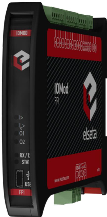
IOMod FPI is a fault passage indicator module for medium voltage applications that can be used as a standalone device or part of Elseta mini RTU with voltages and currents based on sensors technology or with adapters connected to current and voltage transformers with communication support based on Modbus RTU, IEC 60870-5-101, and IEC 60870-5-103 protocols.
